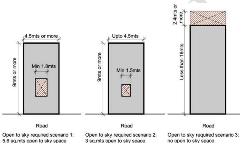
3. In case additional open-to-sky space is provided beyond the minimum requirements, it shall be counted towards the computation of the FSI.
