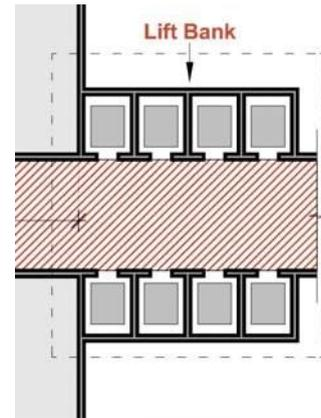
**24.8.2 Lift for Buildings with height more than 25mts:** A lift connecting all floors above ground level shall not continue to the basement. A separate lift shall be required for access to the basement. If, however, common lifts are in connecting with basement, the lift lobby of the basements shall be pressurized, with self-closing door.
