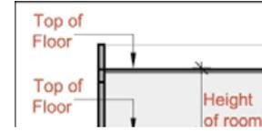
**2. For Industrial Uses,** all occupiable spaces shall have a minimum clearance height of 3.0mts.
