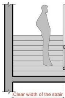
8. **Railing:** Continuous handrails shall be provided on both sides including the wall (if any) at two levels: upper at 850mm–900mm and lower at 700mm to be measured from the base of the middle of the treads to the top of handrails. Floor-mounted railing or parapet shall be provided in such a way that the minimum required width of staircase does not reduce. The maximum gap between balusters shall be 150 mm.
