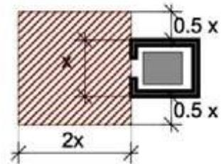
9. The width of the lift landing shall be considered twice the width of the lift well including walls including additional space provided at either side of the landing, and the depth shall be of twice the width of the lift well as illustrated across.
