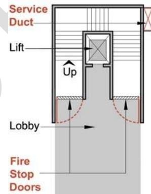
6. No gas piping, electrical panels or AC ducts shall be allowed in the stairway. However service shafts/ ducts may be permitted. Electrical Shafts/ ducts shall have not less than 2hour fire resistance. For other service shafts/ ducts, the fire resistance shall be not less than 1hour.
