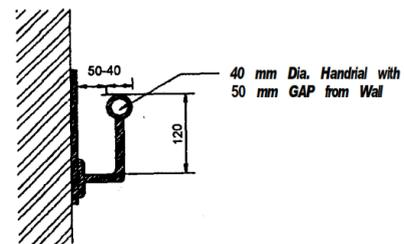
Fixing Detail of Handrail to the Wall
