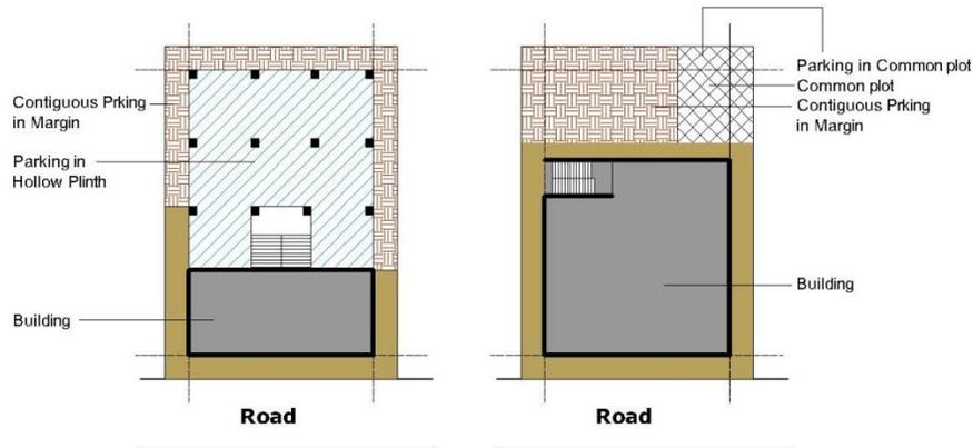
13. **Basement** provided as per Regulation 8.7 shall be permitted within side and rear margins after leaving 3.0mt margin from the boundry of the building unit
