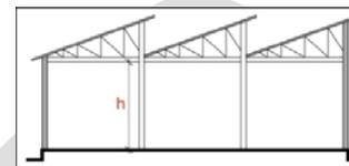
**4. In case of sloping roof, minimum clearance height** shall be 2.2mts (measured from the lowest point of the roof). The average height of the room shall not be less than the minimum clearance height as applicable according to the building use and stipulated above.
