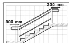
d. Maximum number of risers on a continuous flight without landing shall be limited to 12.
